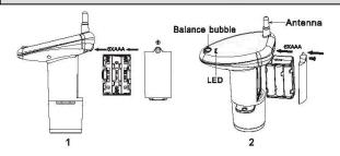
1) Open the battery door, remove the battery box;
