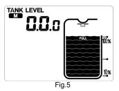
Display of "0.00" and full tank icon flashes (Fig.5). Press +/MAX/MIN key or -/TANK key to increase or decrease air gap. Pressing and holding the keys will change the value at a much faster rate. Press the SET key to save the Air Gap value.
